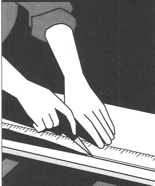
FIGURE 3B- Breaking PLEXIGLAS Sheet*
